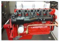
A gentle pressure test at just 2 bar(g), was enough to reassure us that the cracks are fixed, and manifold is ready for use on the engine once more
